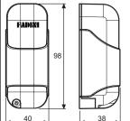
Power supply: 2x1.5AAA or 12V/24V ac/dc Absorption TX: 11mA - 44uA (battery-operated) Absorption RX: 16mA
